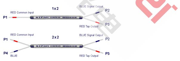
1x2 couplers for blue wavelengths i.e. <500nm are supplied as a 2x2 with an external termination on port P4. 1.
